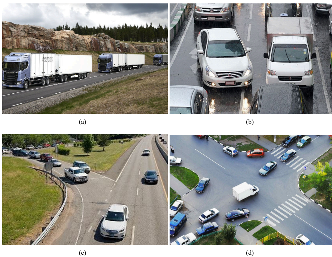
Figure 4. Potential application scenarios for multi-vehicle collaboration. (a) cooperative adaptive cruise of vehicles (adopted from: www.autotrader.co.uk ), (b) cooperative lane changing or merging of vehicles (adopted from: www.roadsafetyuae.com ), (c) merging of vehicles on ramps (adopted from: www.myrecordjournal.com ), (d) cooperative driving at complex intersections (adopted from: https://xsj.699pic.com ).
